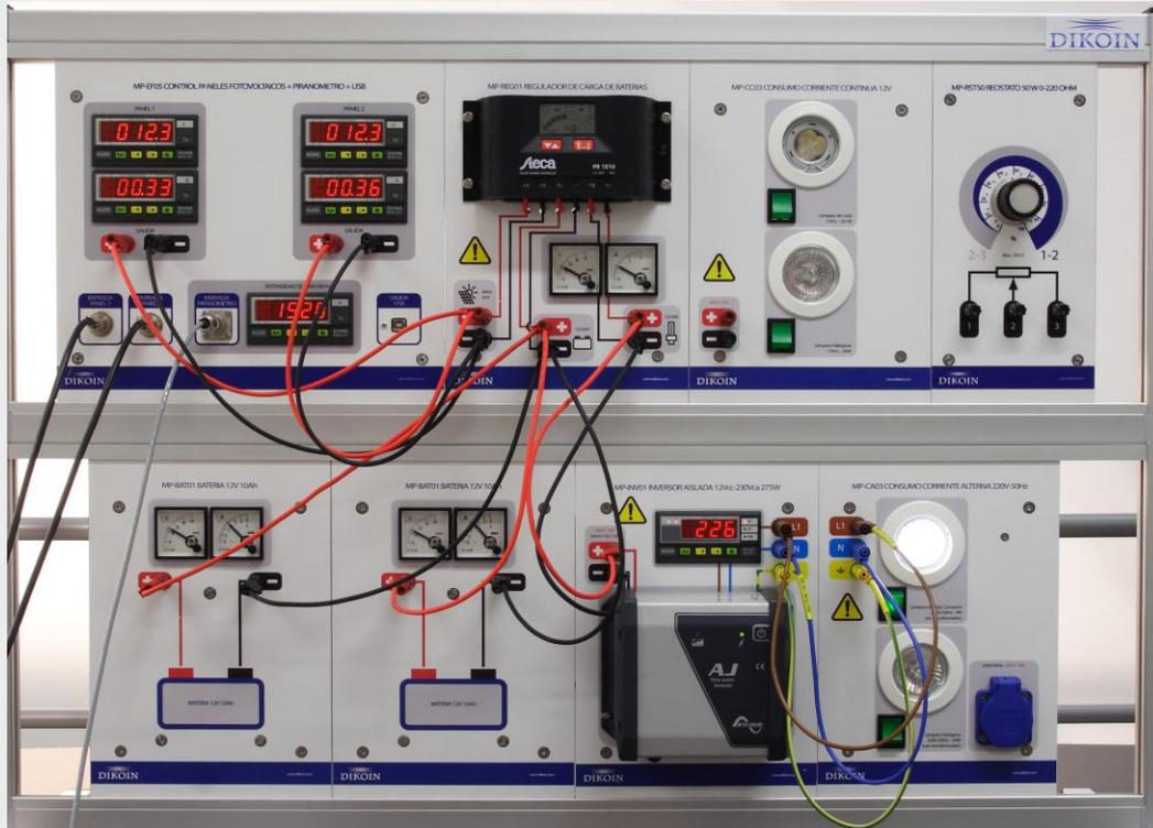
The wiring system through 4mm safety terminals allows a fast and secure connection for the students
