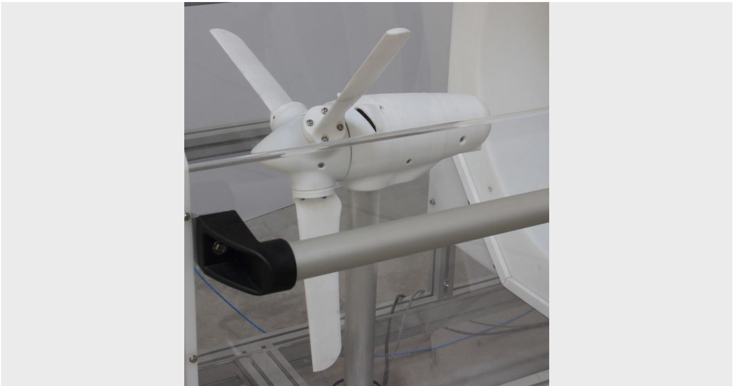
The turbine is fully developed and manufactured by DIKOIN, and has electronic speed and torque measurement systems. It also has an electronic pitch regulation system.
