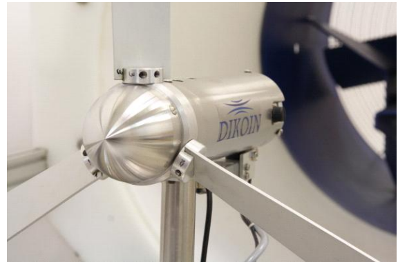
The turbine is fully developed and manufactured by DIKOIN, and has electronic speed and torque measurement systems.
