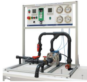
FL 03.2 - CENTRIFUGAL PUMPS CHARACTERISTICS (pag. B - 1)
