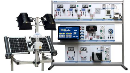
EN 01.6 - COMPUTERIZED PHOTOVOLTAIC INSTALLATION DEMONSTRATOR (pag. E - 1)
