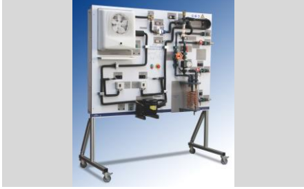
AC 03.1 - HEAT PUMP DEMONSTRATION (pag. F - 1)
