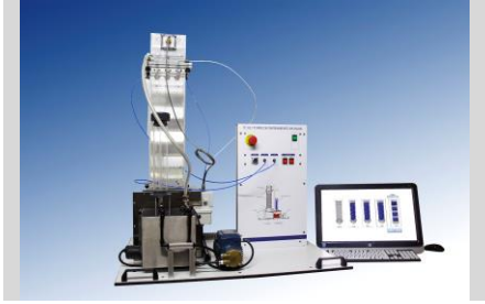
TC 02.1 - WATER COOLING TOWER UNIT (pag. F - 2)
