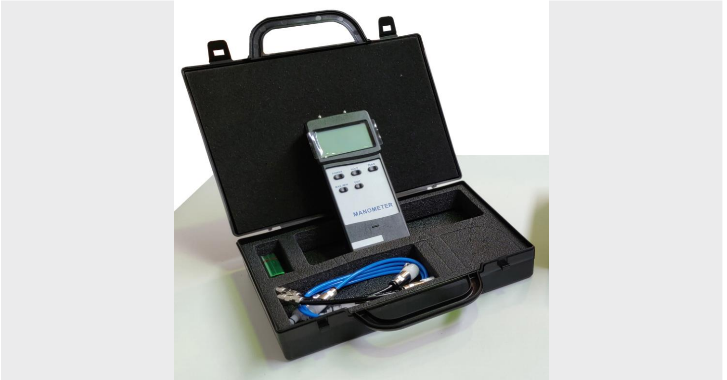
Optional Accessory: FL 01.AC.01 - DIFFERENTIAL ELECTRONIC MANOMETER \pm 7000 mBar WITH QUICK CONNECTIONS Digital differential pressure manometer, used to measure the pressure difference in the suction and impulsion taps of hydraulic pumps, to obtain the characteristic curve of the pump.
