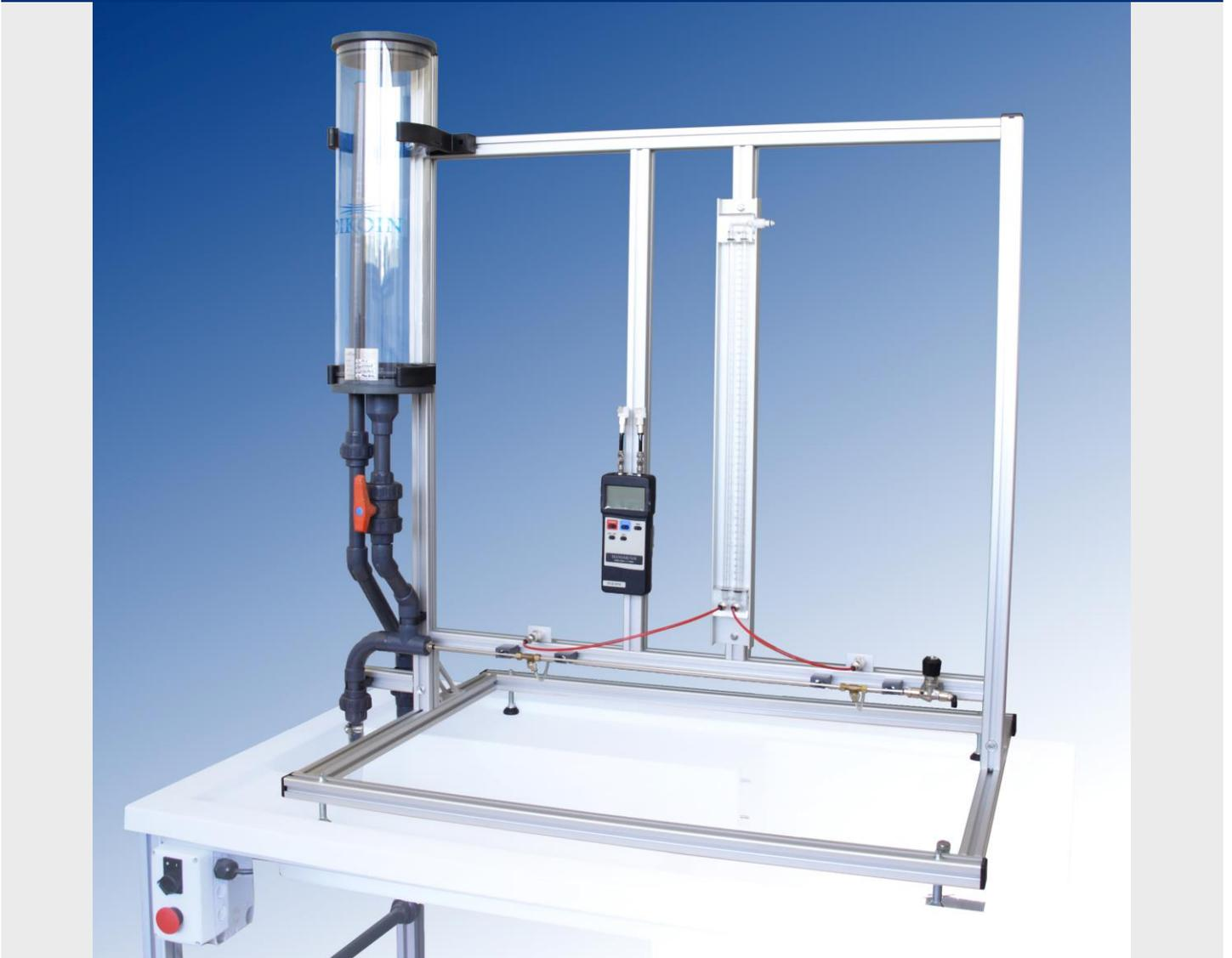
The objective to be achieved with this equipment is the study of primary pressure losses produced along a pipeline in both laminar and turbulent regimen.
