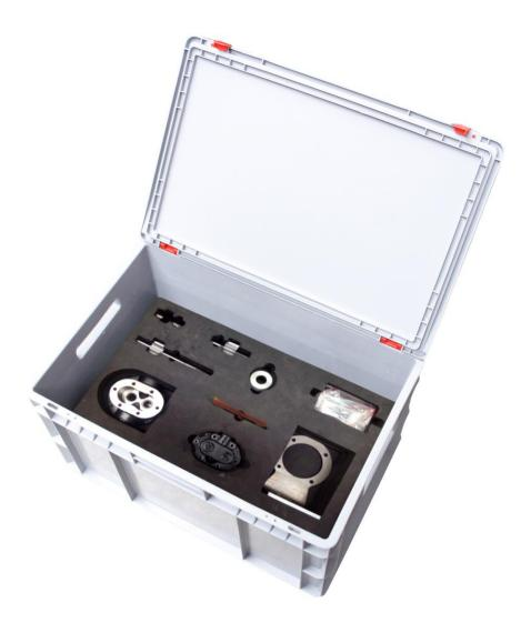
The assembly and maintenance MM07 kit allows the assembly and maintenance of a gear pump. In this type of pumps, the flow rate is proportional to the speed of rotation of the gears (rpm) and with them high pressures and service rates are reached. They are usually used with fluids of high viscosity and free of solid particles. Thanks to the cutting, the student learns all the components of the pump and its operation.
