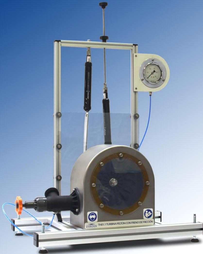
The TH.01.1 equipment simulates an installation in a small scale with a Pelton turbine. It has been designed with special emphasis on the didactic aspect of the same, being able to observe at all times the operation of the system and the different components that constitute it.
