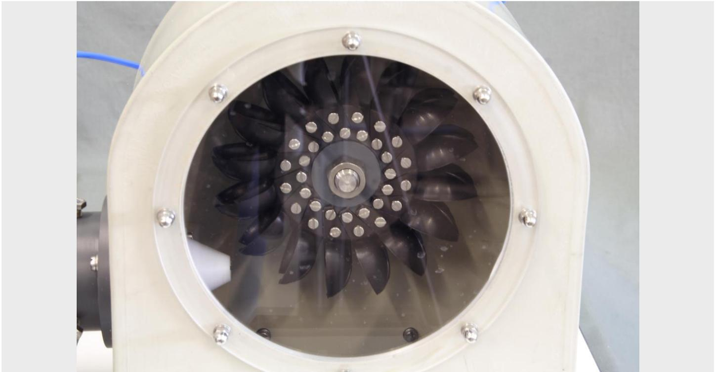
Thanks to its transparent front, you can see perfectly how the water coming out of the injector hits the blades and how, depending on the speed of rotation, the moment the water leaves the blade, in function of the relative velocity of the water relative to that of the impeller.
