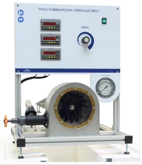
The TH 03.1 equipment simulates a small-scale installation with a Pelton turbine.
