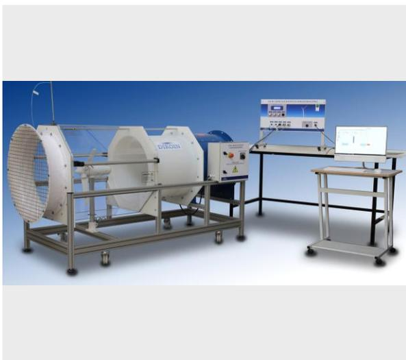
The Windmill Test-bench (EN 04.1), is configured like a wind tunnel of 2 meters length designed to work with windmills of less or equal to 600mm diameter. The equipment has a 600 mm windmill included, which has a torque and rotation speed measurement system connected to the computer, to see real time, the behavior of it.
