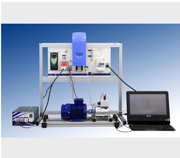
With this equipment the behavior of a windmill is emulated in a practical and didactic way. An electrical motor does the times of the turbine of a windmill to move the DC generator, which transforms the transmitted mechanical energy to the axis into electrical energy.
