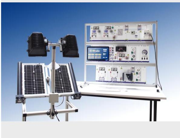
The EN 01.6 equipment scales a complete photovoltaic solar system. It has been designed with special emphasis on the didactic aspect of the same, being able to observe at a glance all the components that a solar photovoltaic installation has and its arrangement. It allows the study, of both isolated photovoltaic solar energy installations and grid connection.
