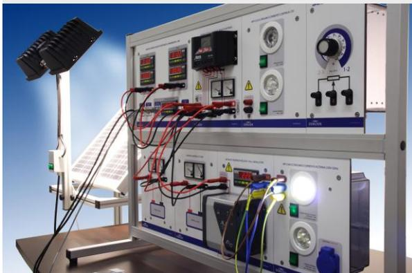
The equipment EN 01.4 is designed like a stand alone photovoltaic solar power plant, with 2 modules and all the elements necessary to complete the installation.
