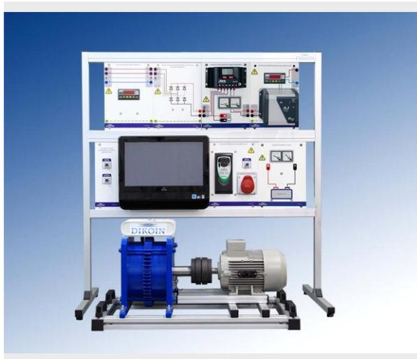
With the EN 04.4 equipment, we emulated the behavior of a wind turbine in a practical and didactic way. An electric motor acts as the blades and bush of a wind turbine, dragging a three-phase synchronous generator of permanent magnets, which transforms the mechanical energy transmitted to the shaft into electrical energy at the output.
