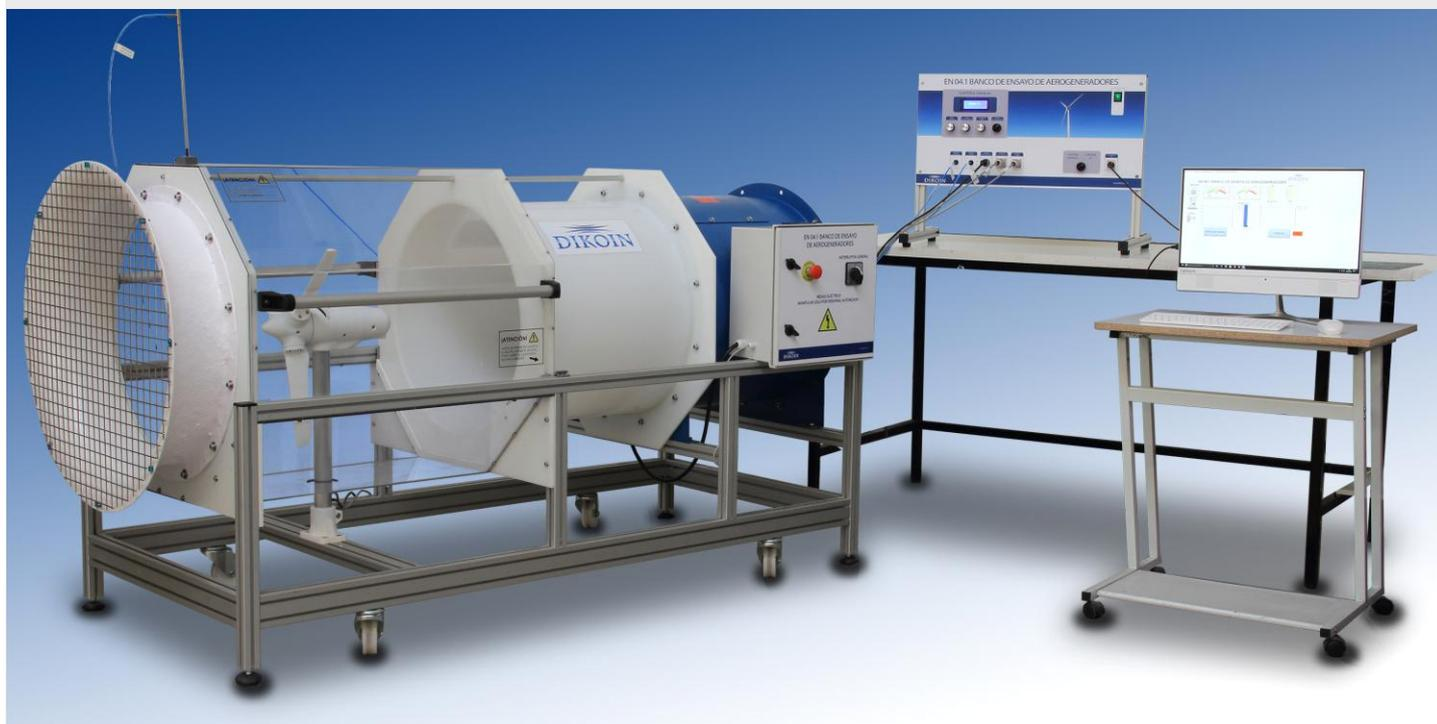
The Windmill Test-bench (EN 04.1), is a wind tunnel of 2 meters length designed to work with windmills of less or equal to 630mm diameter. The equipment has a 612 mm windmill included, which has a torque and rotation speed measurement system.
