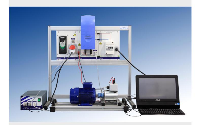
With this equipment the behavior of a windmill is emulated in a practical and didactic way. An electrical motor does the times of the turbine of a windmill to move the DC generator, which transforms the transmitted mechanical energy to the axis into electrical energy.
