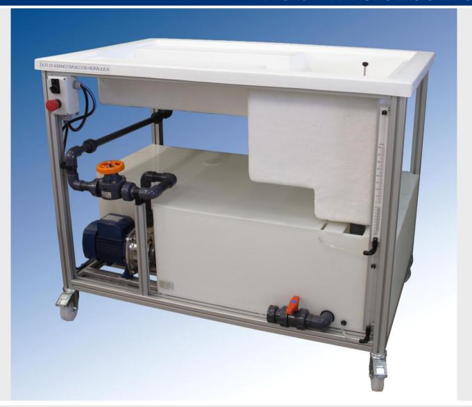
The hydraulic bench is designed as a desk, on which you can use a variety of teaching equipment, in which an input flow needed. It has two volumetric tanks of different sizes, for the measurement of small and large flows with high accuracy.
