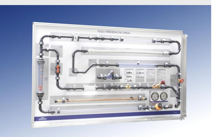
The FL02.1 equipment has been designed for the study of both friction losses in pipes, and the losses of characteristic elements of facilities such as; fittings, valves and measuring elements.
