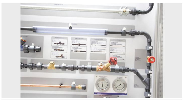
All equipment accessories have a detailed description on foot equipment, allowing easy identification of these and providing information at the time of calculation of pressure drop in each and everyone of the accessories.
