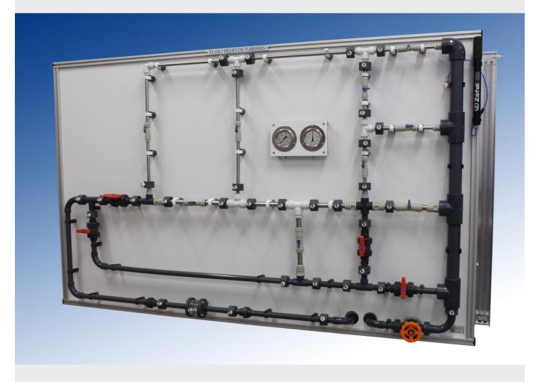
The pipeline networks equipment FL 04.1 has been developed for the study and analysis of the flow through pipe networks. During the design we've thought on a complete and flexible equipment, so that the user can study the higher possible number of configurations and as complex or simple as they wish.
