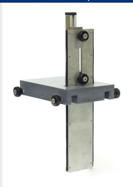
Included Accessory: HD.Z.11 - VERTICAL GATE (For Flow channel) Vertical gate for hydrodynamic channel.
