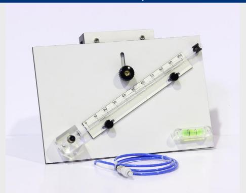
Optional Accessory: HD.Z.02 - INCLINED MANOMETER Inclined manometer to flow channel.
