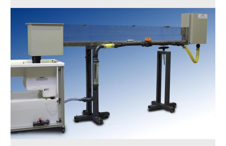
This equipment is designed to study the behavior of fluids in open channels by conducting a wide range of practices and experiences.
