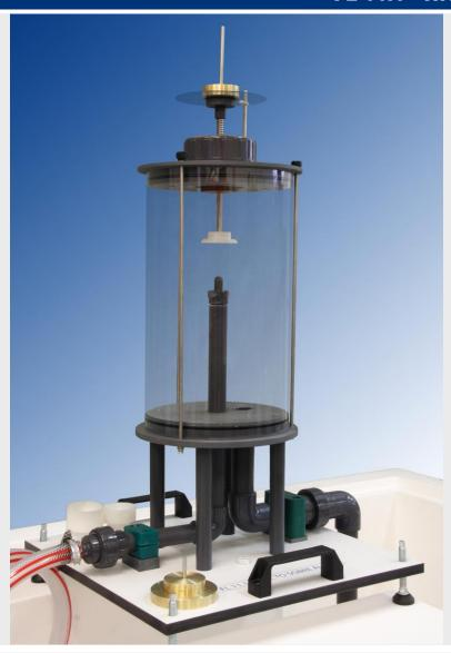
This equipment has been designed to verify the validity of the theoretical expressions that determine the force exerted by a jet on different types of blades.
