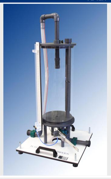
The FL12.1 equipment has been designed for the study of everything related to the phenomenon of contraction that occurs when a jet of fluid passes through a orifice. It has been designed with special emphasis on its didactic use and that is why the equipment has three nozzles whose geometry differ between them, being able to perform tests in different conditions, facilitating to the student the compression of the phenomenon that is produced.
