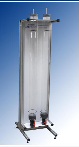
This equipment has been designed for the determination of the viscosity of several liquids, and the study and verification of the resistance coefficients of various geometric shapes.
