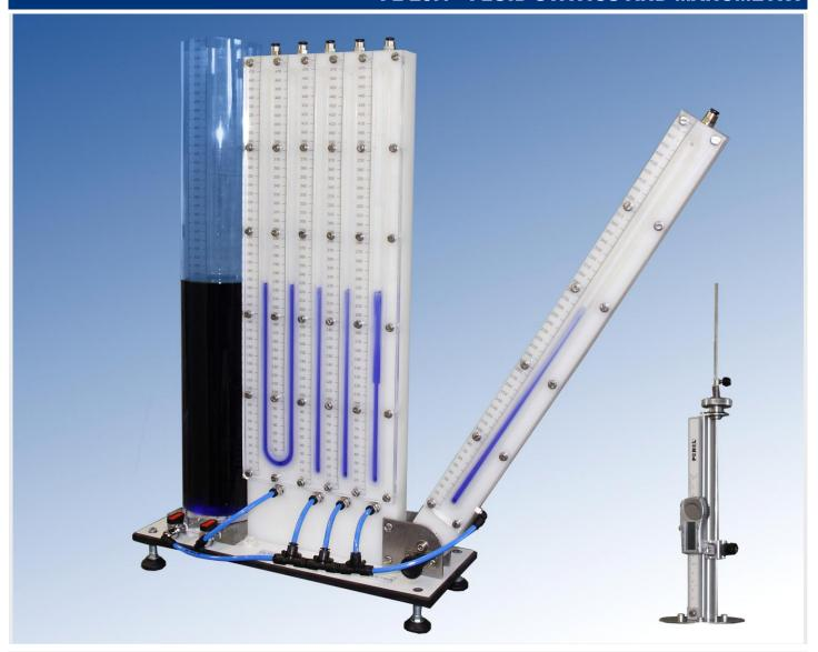
Equipment designed for the study of fluid static and pressure measurement with different types of piezometric tubes and level measuring elements such as graduated scales and limnimeter.
