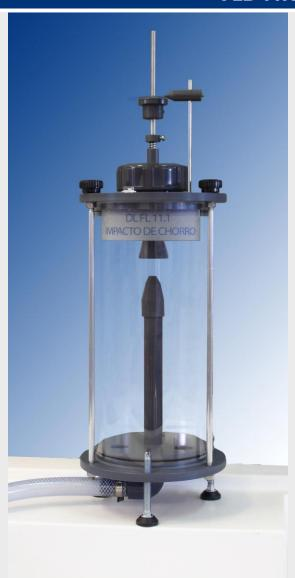
This equipment has been designed to verify the validity of the theoretical expressions that determine the force applied by a jet stream on different types of deflectors.
