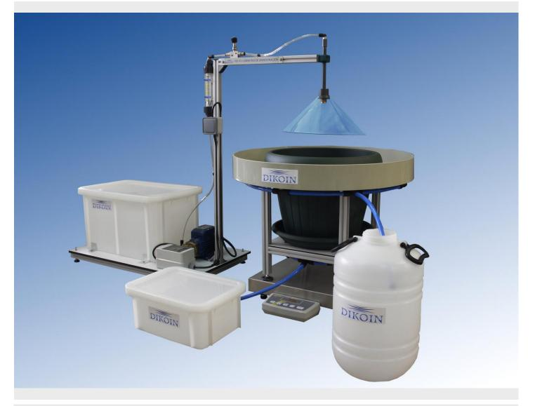
With the HD 10.1 equipment, it is a question of knowing the water retention capacity of a soil using the hydrological balance, differentiating each one of its elements.
