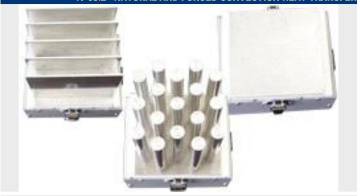
The equipment is supplied with 3 different heat transfer surfaces: Flat plate, finned and pinned.
