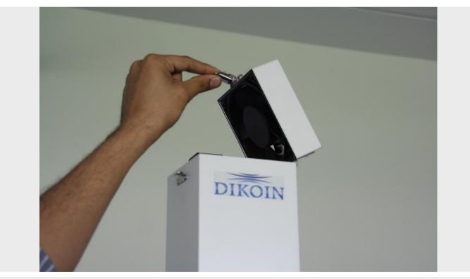
The system of decoupling the fan by fast anchorage and hinges, allows that in the study of natural convection, the duct is totally free of all obstacles, so that the calculation of convection is much more precise.
