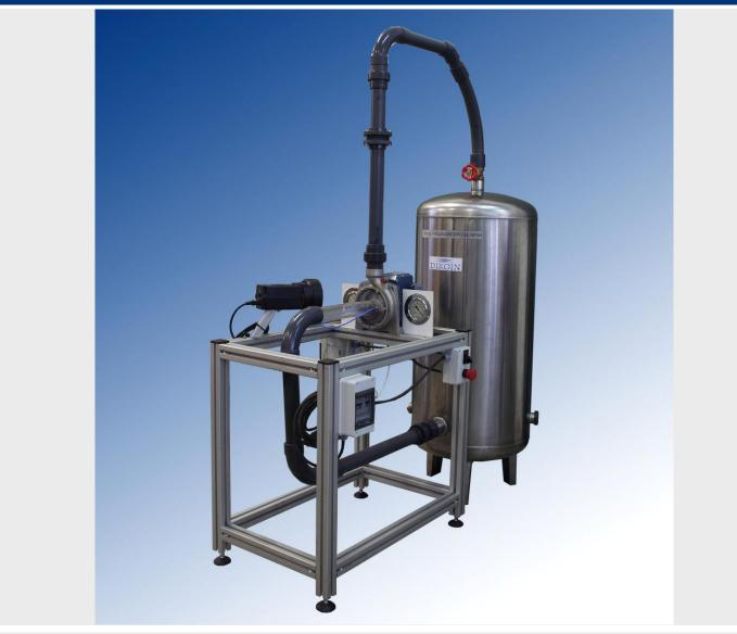
Cavitation is produced when a liquid that is being pumped loses pressure and matches the level at which vapour is generated at the same temperature the pump is operated. At that moment, liquid turns into vapour, giving rise to vapour locks or vacuum pockets that are pushed into other areas with a higher pressure. Very fast condensation takes place creating short-lived excess of pressure in very small places.
