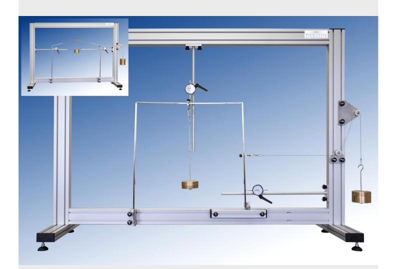
The objective of this equipment consists on the study of the deformation in the plane, of frame type structures under the action of solicitations. The equipment is supplied with a gantry in U and another with a "gable" roof.
