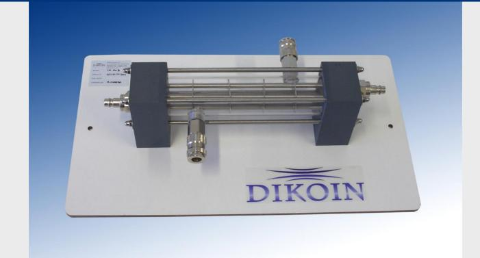
Optional Accessory: TC 01.3 - SHELL TUBE HEAT EXCHANGER The beam exchanger tubes is one of the most used in industry exchangers.
