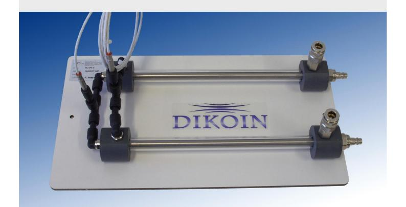
The concentric tube heat exchanger is the simplest in design among all the heat exchangers.
