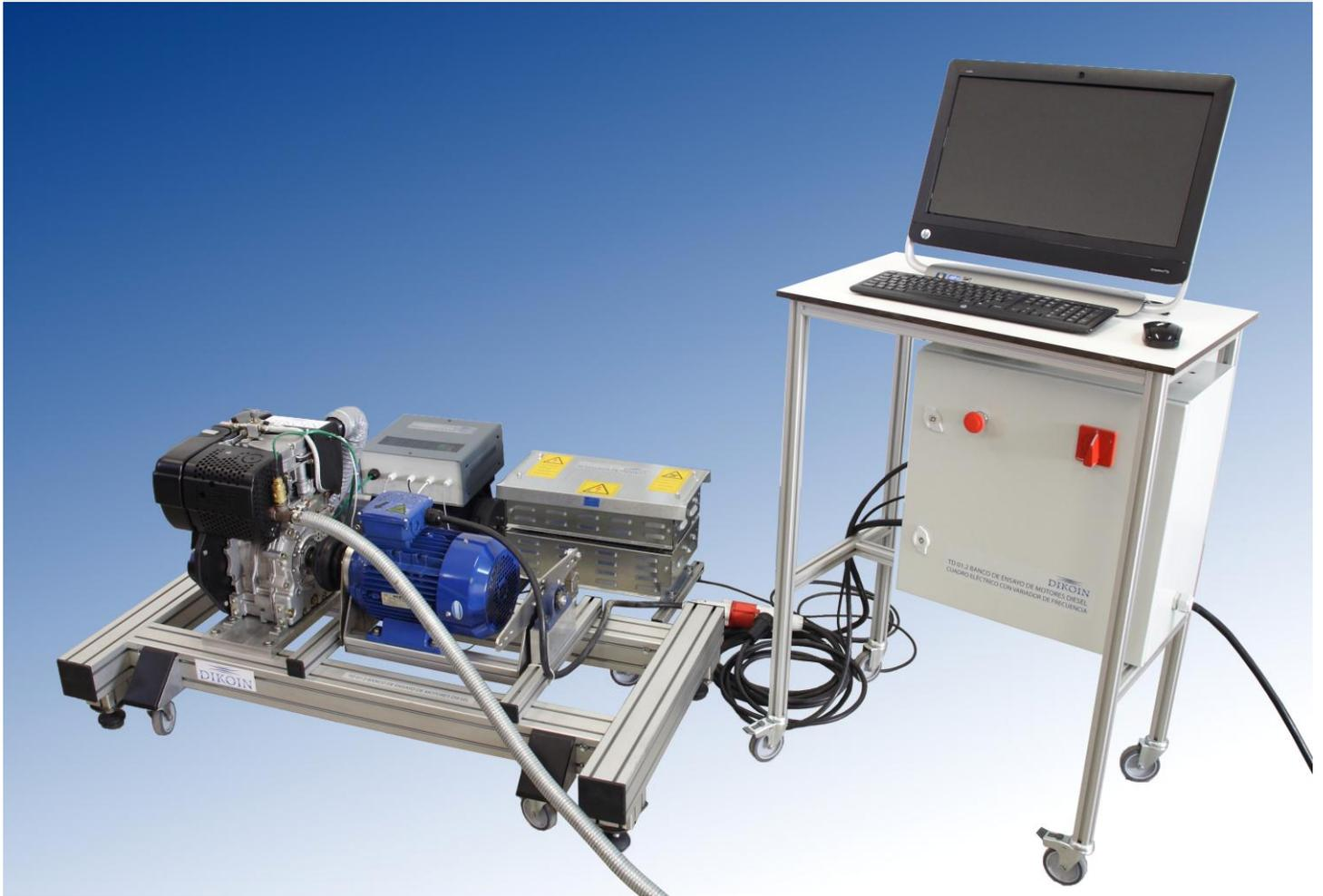
Equipment designed for the study and understanding of the behavior of a four-stroke single cylinder diesel combustion engine.
