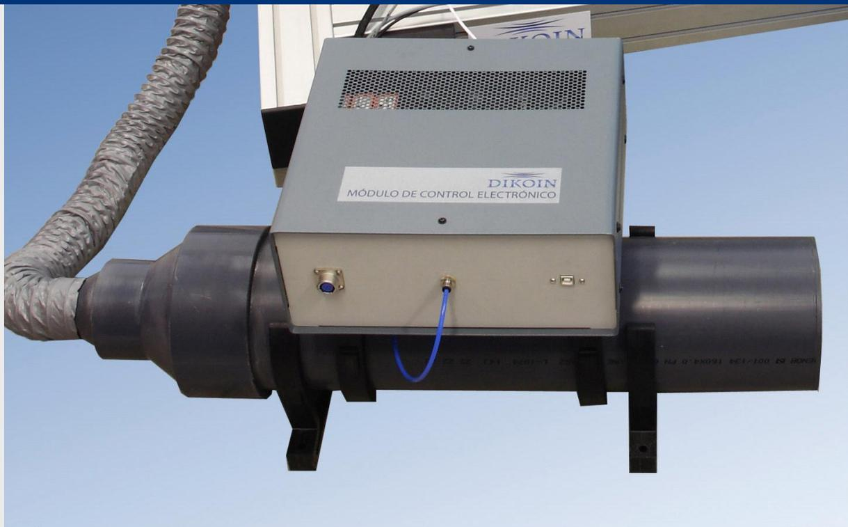
The system has a device for measuring the volume of air sucked by the engine, so that calculations can be made corresponding to the air-fuel ratio, etc.
