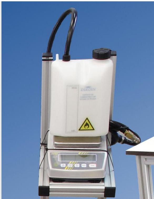
In order to measure the amount of fuel consumed as accurately as possible, we have designed a weighing system.
