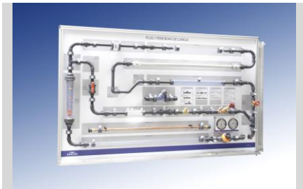
FL 02.1 - LOSSES IN PIPES PANEL (pag. A - 3)
