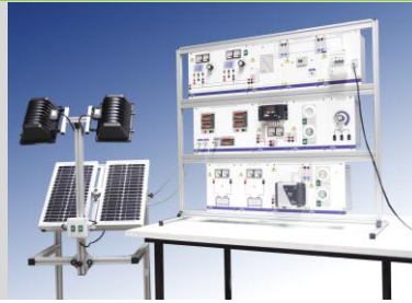
EN 01.5 - STAND ALONE AND NETWORK CONNECTED PHOTOVOLTAIC INSTALLATION DEMONSTRATOR (pag. E - 1)
