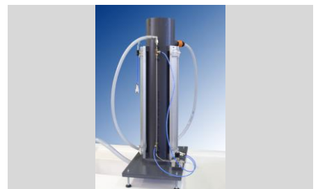
FL 17.2 - LOSSES IN PIPES (pag. A - 9)
