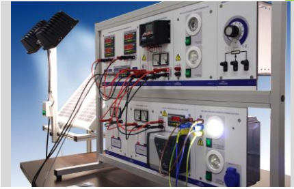
EN 01.4 - STAND ALONE PHOTOVOLTAIC INSTALLATION DEMONSTRATOR (pag. E - 1)
