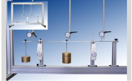
ST 03.1 - CONTINUOUS BEAMS (pag. K - 1)
