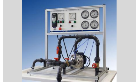
FL 03.2 - CENTRIFUGAL PUMPS CHARACTERISTICS (pag. B - 1)
