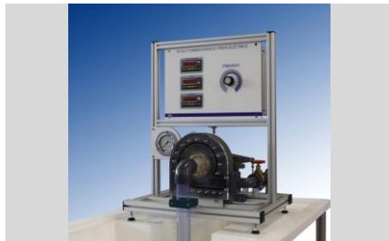
TH 03.2 - ELECTRIC BRAKE FRANCIS TURBINE (pag. B - 4)
