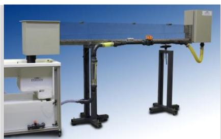
FL 05.5 - CANAL HIDRODINÁMICO PARA BANCO HIDRÁULICO 2,5M (pag. C - 2)
