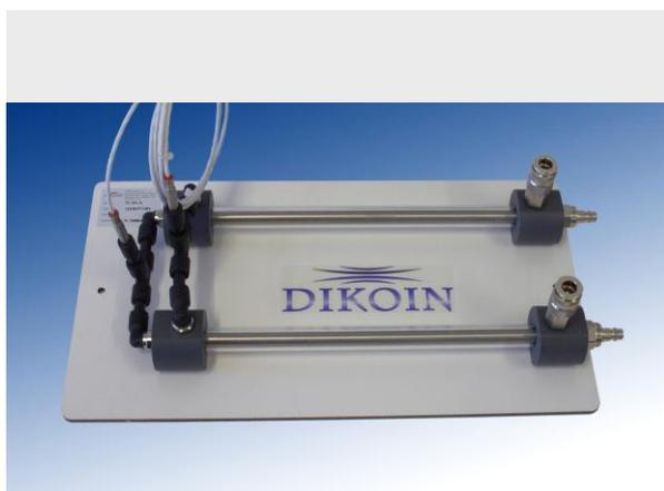
The heat exchanger of concentric tubes is simpler in design.
