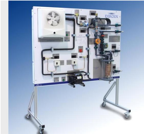
The AC 03.1 equipment demonstrates clearly the operation of a heat pump air / water.
