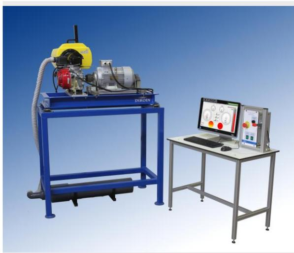
The TD 01.1 equipment, has been designed for the study and understanding of the behavior of a gasoline four-stroke combustion engine.
