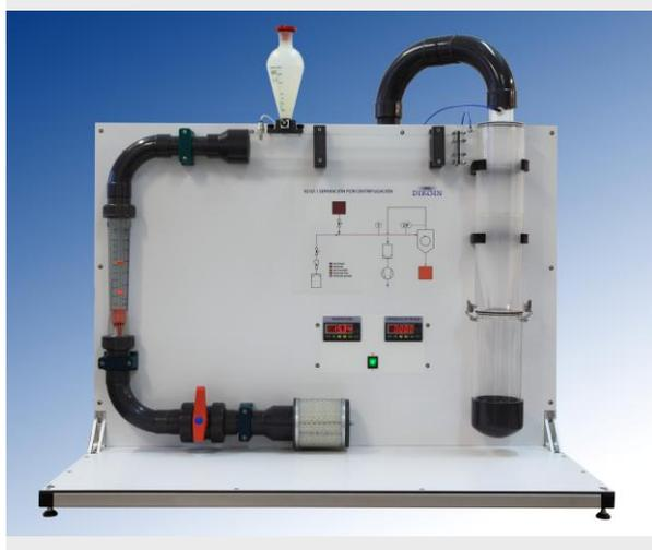
Cyclones are widely used equipment in the industry that allows the separation by centrifugal force of solid particles that are suspended in a gas. They are simple equipments whose operation is based on the separation of the particles by means of the centrifugal force, and that without having movable parts they have a very simple maintenance. As inconvenience we can emphasize that they are not flexible to the changes of concentration, flow or size of the particles.
