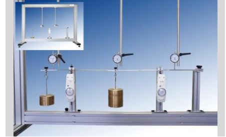
ST 03.1 - CONTINUOUS BEAMS (pag. K - 1)
