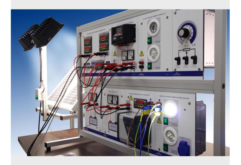
The equipment EN 01.4 has been designed as a stand alone photovoltaic solar power plant, with 2 modules and all the elements necessary to complete the installation.
