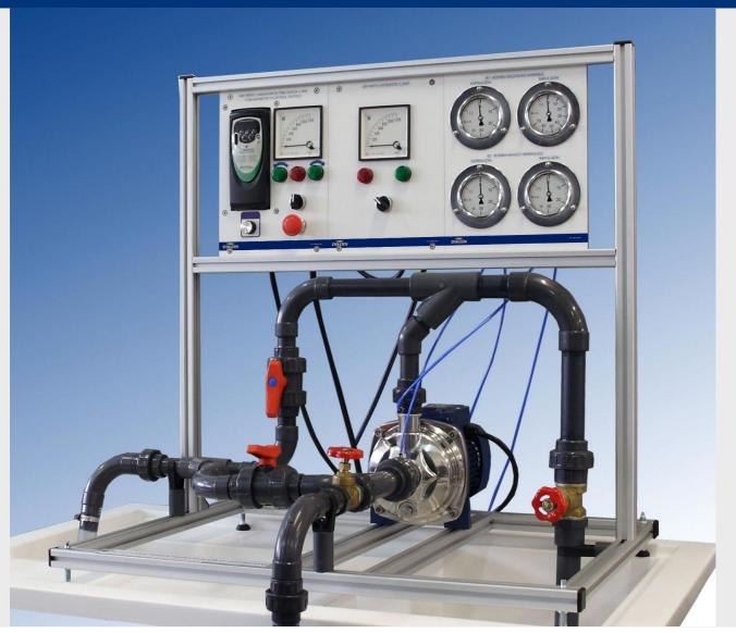
The equipment is designed to operate on hydraulic bench. The installation is mounted on a frame constructed of aluminum, with a system of pipes and valves that allow it to be coupled hydraulic pump and bank equipment in series or in parallel.
