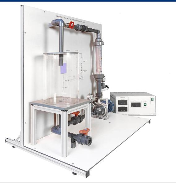
The Centrifugal Pump Demonstration unit makes it possible to carry out a range of operations, either for the start-up or the operation itself of a pump station. The study of how a single pump works is available through the following coursework and laboratory experiments:
