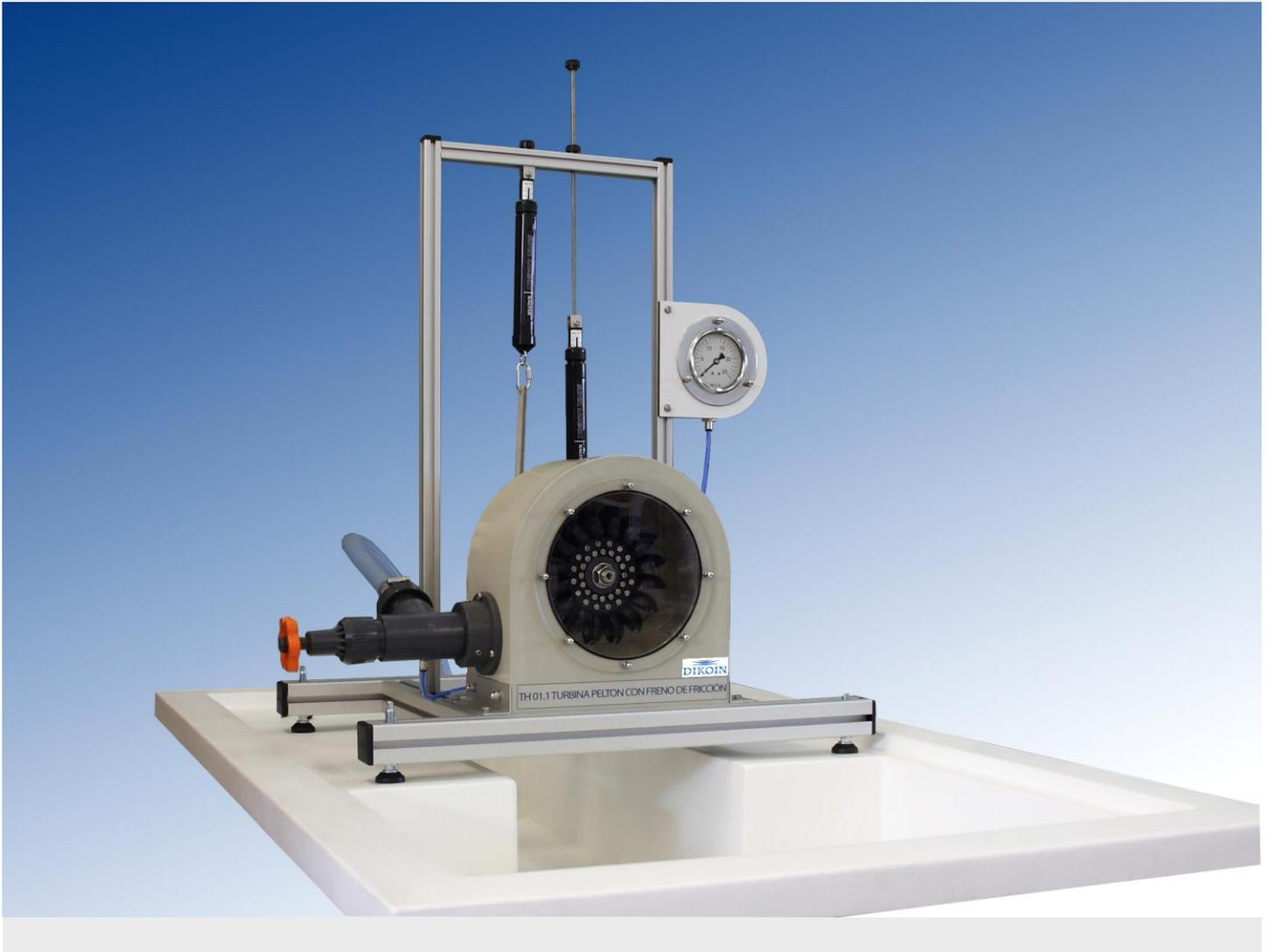
The TH.01.1 equipment simulates an installation in a small scale with a Pelton turbine. It has been designed with special emphasis on the didactic aspect of the same, being able to observe at all times the operation of the system and the different components that constitute it.
