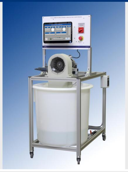
The TH 04.1 equipment simulates a small-scale installation with a Pelton turbine.
