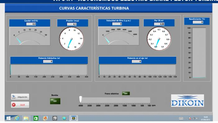
The equipment includes a PC with the equipment management software. In which the parameters of all control points of the equipment are shown, and the data collection is allowed in automatic or manual mode.
